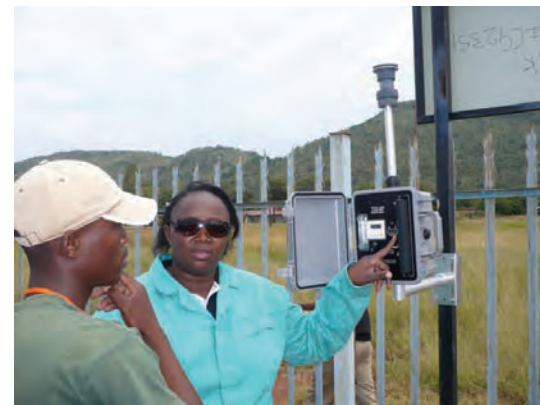
Monitoring air quality, March 2009. Small dust particles can cause serious breathing problems. This PM10 monitor measures dust particles that are less than one tenth of a millimetre in size. Wesizwe has to keep the dust produced by its activities to a minimum.
